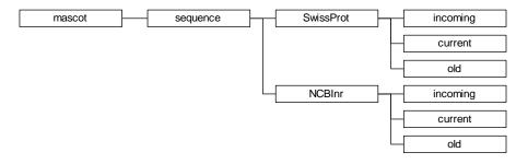
For each database, the *incoming* directory provides a workspace for downloading and expanding a new database file. The *current* directory contains the active database, and this is where Mascot Monitor creates the memory mapped compressed files. The *old* directory is where the immediate past database file is archived ... just in case.
